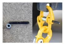
**Step 3.** Bring the two halves of the links together and partially insert locking pin to hold the parts together.
