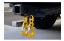
When using two chains, repeat the process on the other hitch point of the tow bar.
