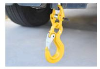
**Step 4.** Insert the locking collar with the recessed side facing the pin and push the pin in until it holds the collar in place.
