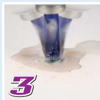
Make a swinging movement to allow for dust evacuation.
