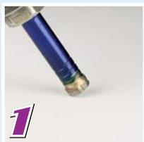
Water the drilling area. To avoid drill slipping start with a 45° angle.
