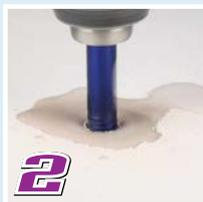
After the hole is started gradually straighten up the drill.
