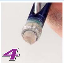
Make sure the core has been removed from bit after drilling.
